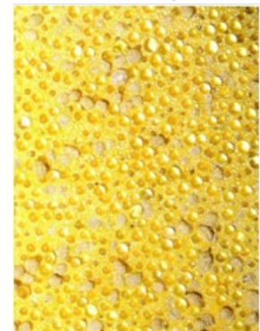
Exhibit 26: Closeup of Recess Triple Drop pavement marking, with glass beads and ceramic elements
