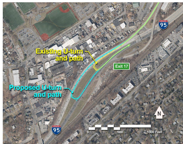
Exhibit 17: Existing and proposed U-turns and vehicle paths for emergency response vehicles
