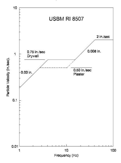
Figure 1—Safe Vibration Limit Recommendations for Residential Structures
